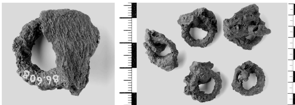
Fig. 4. On the left – one of the five iron rings 86.608 with a piece of hide. This was used for the SEM examinations. On the right – all five rings.
