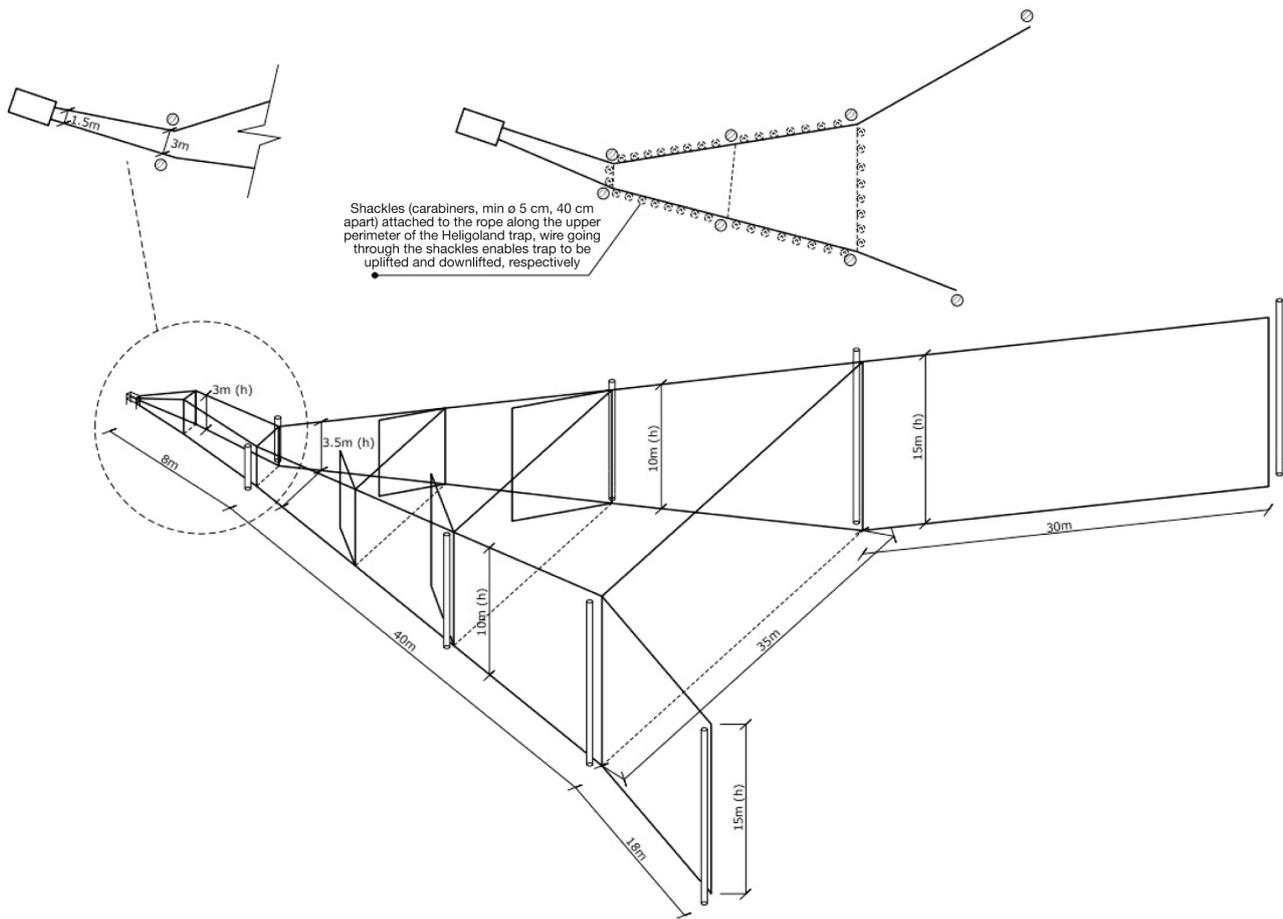
Fig. 2. Scheme of the trap build in Pape in 2014 for bat trapping (drawing by Reinis Priedols).
